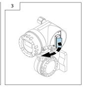
Make a note of the terminal assignment, as this makes for easier connection following installation later on.
