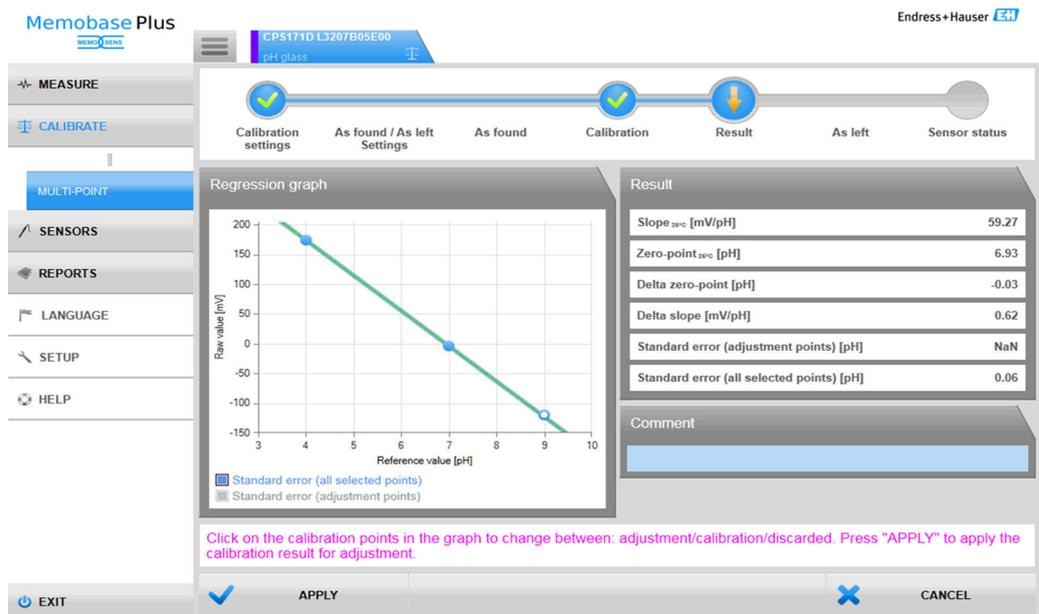
**16** Multipoint calibration: buffers 4 and 7 selected as the adjustment points, buffer 9 as the calibration point
