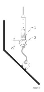
In order to prevent an extremely high tensile strength (e.g. due to thermal expansion) and the risk of the rope breaking, the rope has to be slack. Minimum sag (A):  $\geq$  10 mm/(1 m rope length) [0,12 in/(1 ft rope length)].
