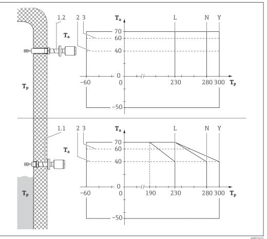
Device type FTL70, FTL71, Basic specification, Position 11 (Application) = L, N, Y
