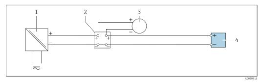
■ 17 Connection example for 4 to 20 mA current input
