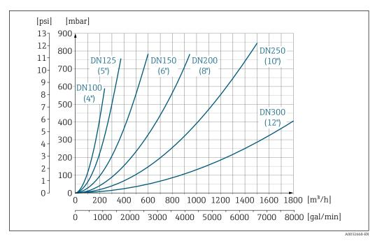
35 Pressure loss DN 100 to 300 (4 to 12") for order code for "Design", option C "fixed flange, without inlet/outlet runs"
