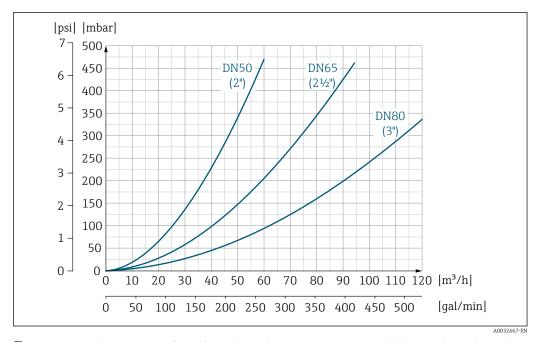
234 Pressure loss DN 50 to 80 (2 to 3") for order code for "Design", option C "fixed flange, without inlet/outlet runs"
