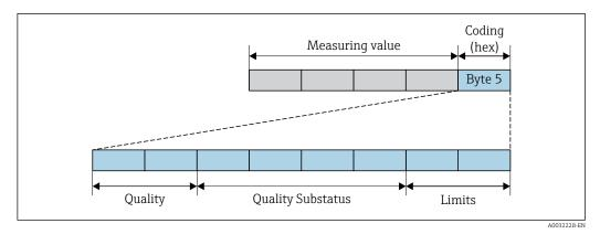
■ 29 Structure of the coding byte
