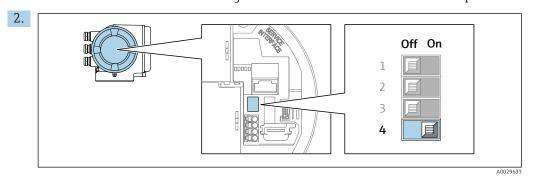
To switch addressing from software addressing to hardware addressing: set the DIP switch to  ${\bf On}$ .
