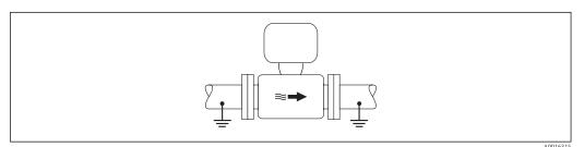
$\blacksquare$  8 Potential equalization via measuring tube
