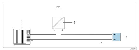
16 Connection example for relay output (passive)
