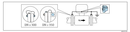
$\blacksquare$  9 Potential equalization via ground terminal and pipe flanges
