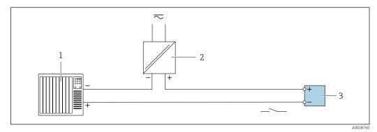
■ 15 Connection example for switch output (passive)
