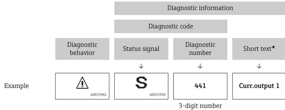
If two or more diagnostic events are pending simultaneously, only the message with the highest priority is shown. Other diagnostic messages that are pending can be viewed in the **Diagnostic list** submenu →
