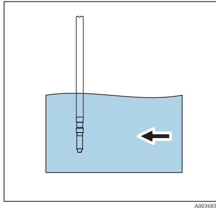
The installation angle is 0°. The arrow indicates the flow direction; it runs from the 10 mm (0.39 in) path to the 5 mm (0.2 in) path. If the sensor is used in open basins, install the sensor in such a way that air bubbles cannot accumulate on it.
