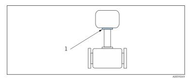
Position of reference point for temperature measurement
