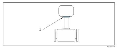
I Position of reference point for temperature measurement
