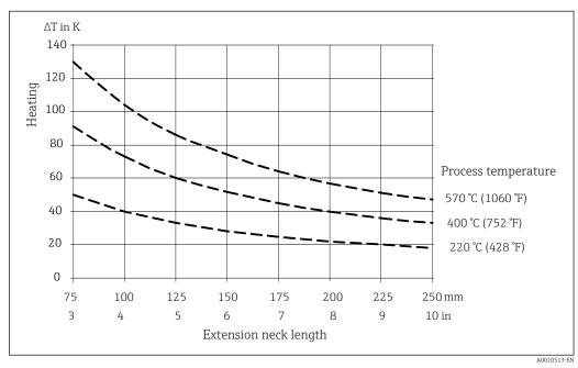
■ 6 Heating of the terminal head as a function of the process temperature. Temperature in terminal head = ambient temperature 20 °C (68 °F) +  $\Delta T$
