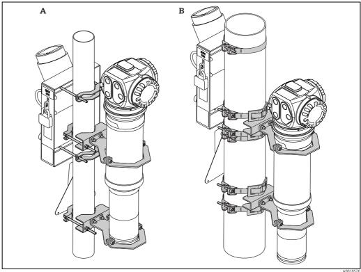
Clamping device for pipes with outer diameters 48 to 77 mm (1.89 to 3.03 in) Clamping device for pipes with outer diameters 80 to 273 mm (3.15 to 10.7 in)
