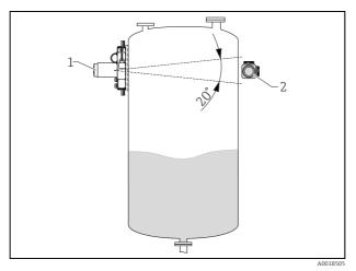
For level limit detection, the radiation source container is mounted at the same height as the detector.
