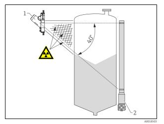
A distance between the source container and the product vessel often cannot be avoided if the measuring range is large and the container diameter small. This space must then be blocked off and marked.
