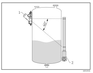
The source container must be mounted at the height of, or slightly above, the maximum level for continuous level measurement. The radiation must be aligned exactly with the compact transmitter mounted opposite. The source container and compact transmitter should be mounted as close as possible to the product vessel to avoid control zones.
