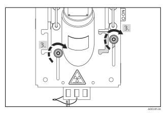
3. Tighten the clamps again. Perform the recalibration.
