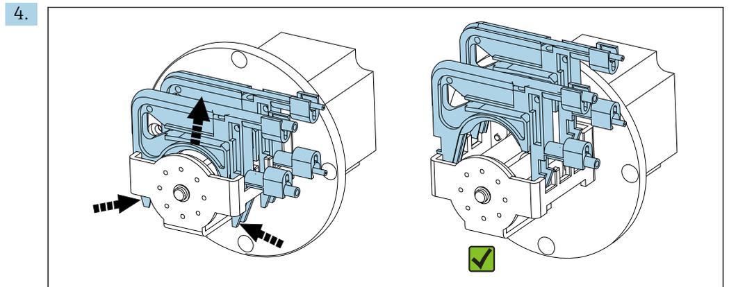
**20** Hose cassettes (pump P1: sample hose at front, condensate hose at rear)
