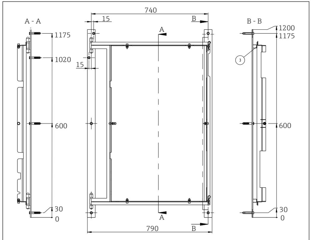
6 Pivoting frame for wall mounting, dimensions in mm (inch)
