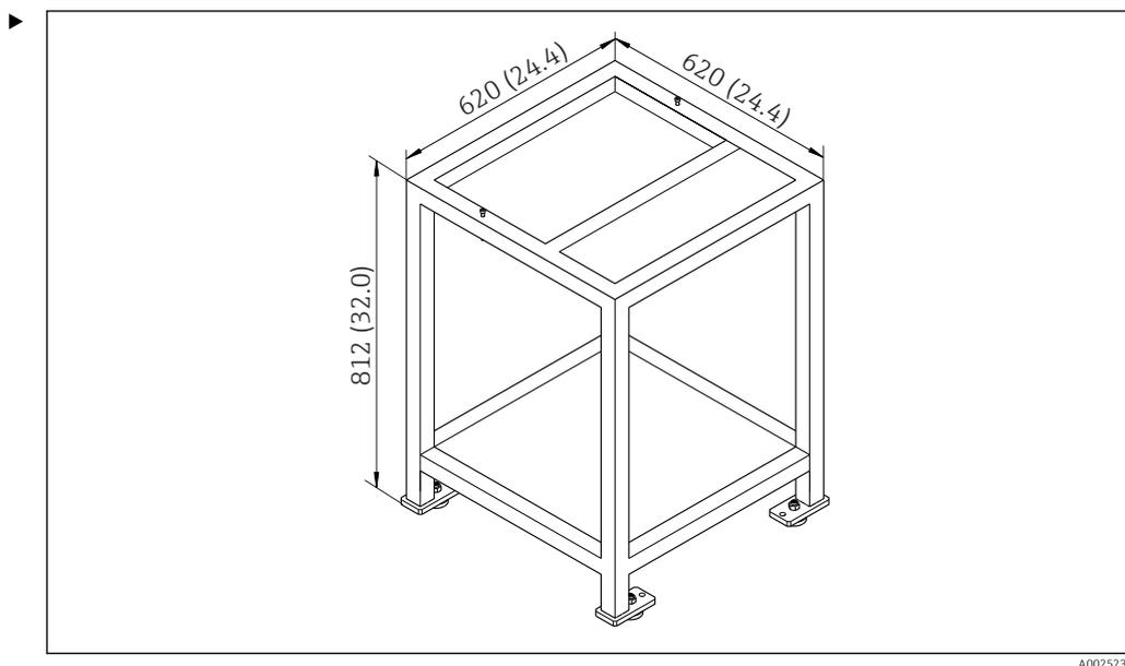
7 Mounting on a base frame in mm (in), height without height-adjustable feet
