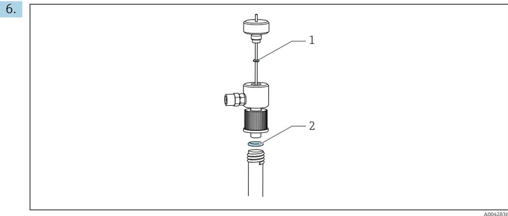
Check the O-rings (1 only if replacing the capillary).
