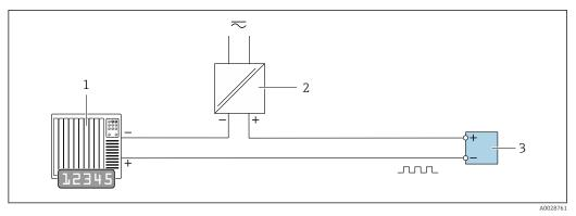
12 Connection example for pulse/frequency output (passive)
