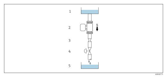
• 4 Installation in a down pipe (e.g. for batching applications)
