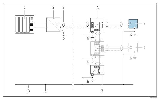
Connection example for FOUNDATION Fieldbus
