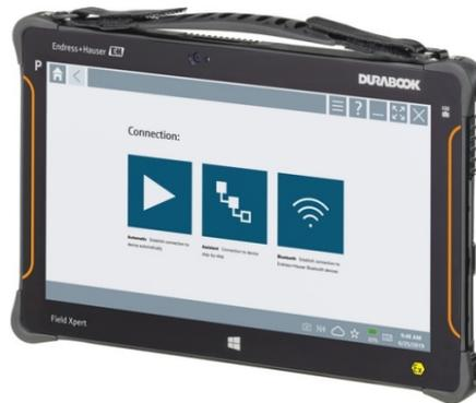
**Figure 2.4: Field Xpert SMT70 industrial tablet**
