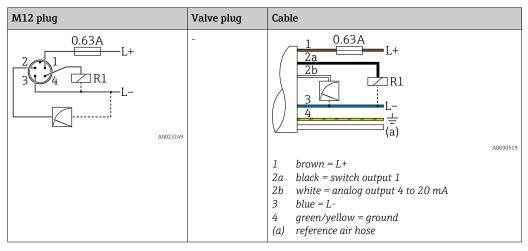
IO-Link: 1 x PNP switch output R1 with additional analog output 4 to 20 mA (active)
