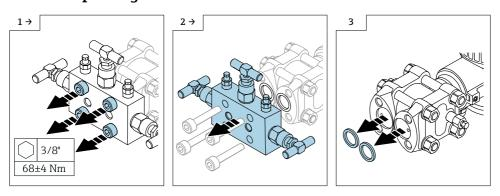
Installation is performed by following the removal procedure in reverse order.
