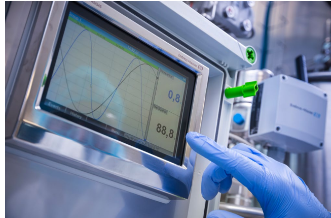
Memograph M RSG45 advanced data manager with stainless steel housing for sterile applications
