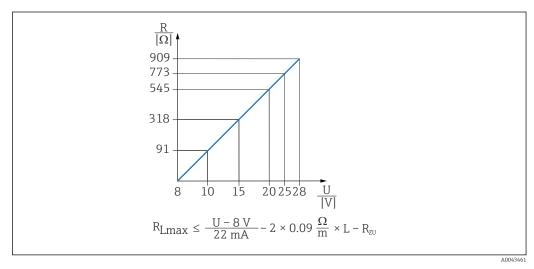
$R_{Lmax}Max$ . Bürdenwiderstand  $[\Omega]$
