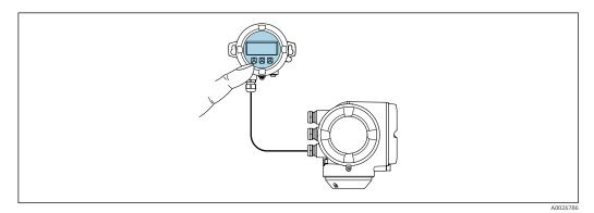
$\blacksquare$  36 Operation via remote display and operating module DKX001
