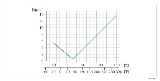
$\blacksquare$  33 Field density calibration, for example at +20 °C (+68 °F)
