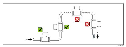
To prevent measuring errors arising from accumulation of gas bubbles in the measuring tube, avoid the following mounting locations in the pipe:
