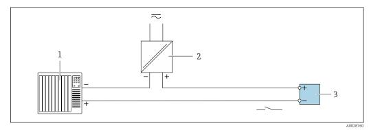
■ 16 Connection example for relay output (passive)
