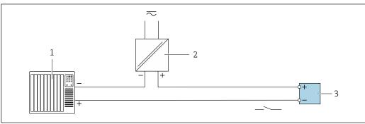
15 Connection example for switch output (passive)
