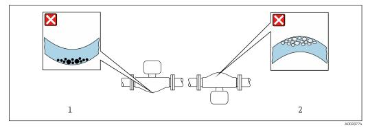
■ 6 Orientation of sensor with curved measuring tube
