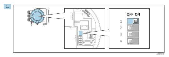
Setting the write protection (WP) switch on the main electronics module to the **ON** position enables hardware write protection.
