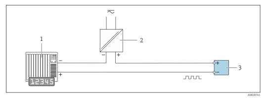
■ 13 Connection example for pulse/frequency output (passive)
