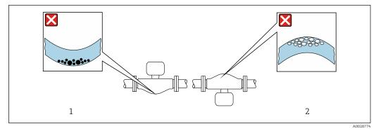
$\blacksquare$  5 Orientation of sensor with curved measuring tube
