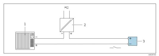
■ 15 Connection example for relay output (passive)
