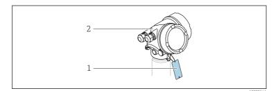
Isolated capacitance: with one metal plate: ≤ 3 pF (permitted in all areas for Equipment Groups II and III) with two to three metal plates: ≤ 10 pF (not permitted in Zone 0 and for Equipment Group IIC)
