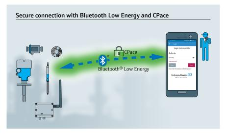
Currently all Endress+Hauser measuring instruments with Bluetooth® connection are supported
