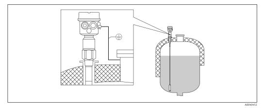
A probe with inactive length for the insulated tanks
