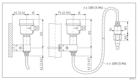
Housing side: wall mounting, pipe mounting, and sensor side. Unit of measurement mm (in)
