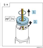
Remove the seal and loosen the adapter disk with the open-end wrench AF34.
