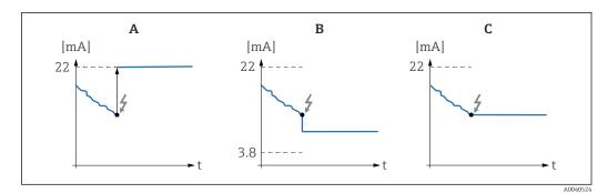
A Output current flow in "Max" setting
