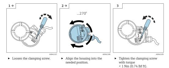
The clamping screw for aligning the housing type T13 is located in the electronics compartment.
