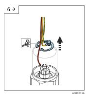
Remove the snap ring with a snap ring pliers.
