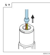
Pull out the cable with the cone.
