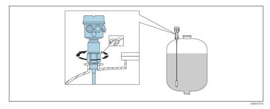
1. Screw the probe onto the proper place.
