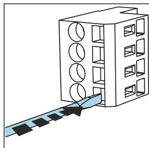
14 Press the screwdriver against the clip (opens the terminal)
