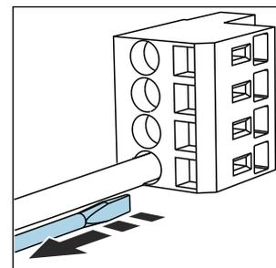
16 Remove the screwdriver (closes the terminal)
