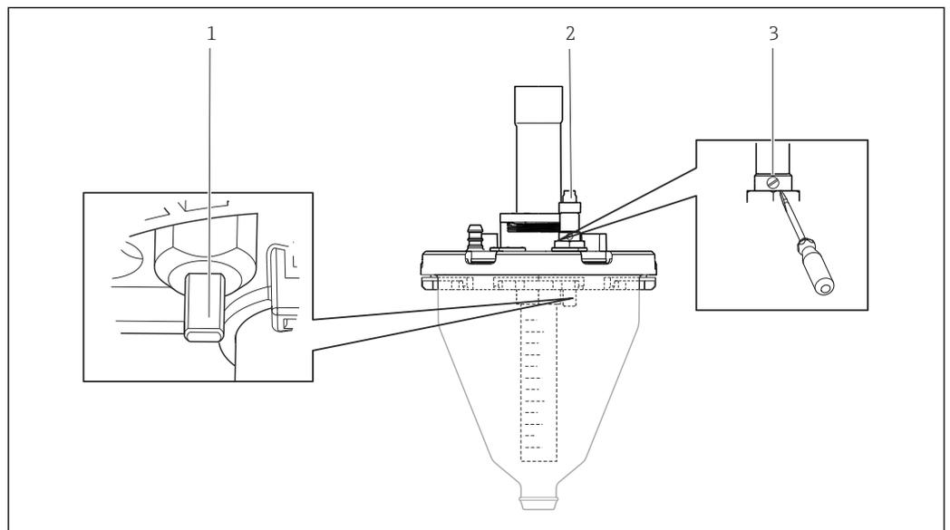
**43** Capacitance sensor adjustment
