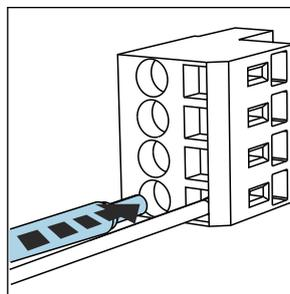
15 Insert the cable until the limit stop
