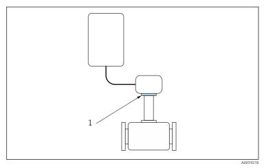
I Position of reference point for temperature measurement
