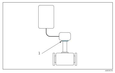
■ 1 Position of reference point for temperature measurement
