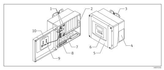
• 1 Parts of the Prosonic S in the polycarbonate field housing
