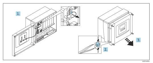
For easier wiring, remove the cover from the field housing
