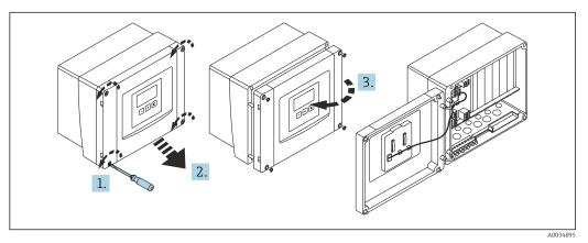
I6 Access to terminal compartment in polycarbonate field housing
