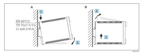
🖻 12 Mounting/disassembling the DIN rail housing. Unit of measurement mm (in)
