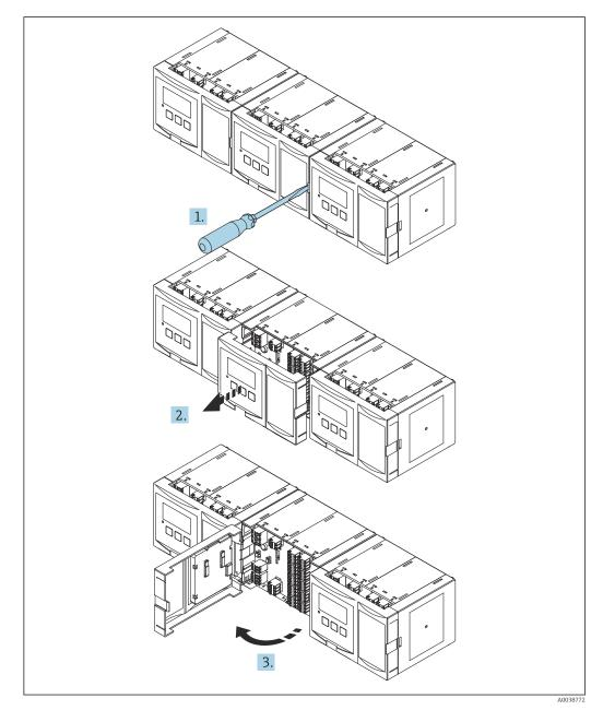
■ 20 Access to terminal compartment: several DIN rail housing units mounted side by side
