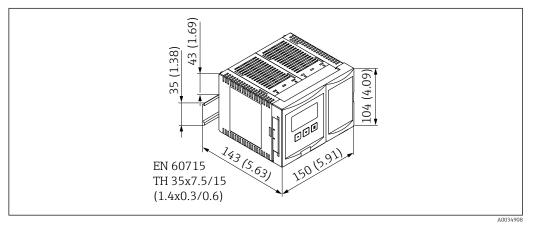
■ 11 Dimensions of Prosonic S with DIN rail housing. Unit of measurement mm (in)
