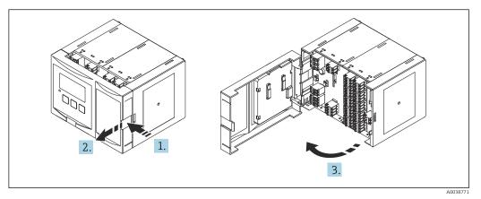
🖲 19 Access to terminal compartment: single DIN rail housing unit
