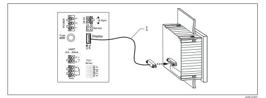
■ 32 Connection of the remote display and operating module
