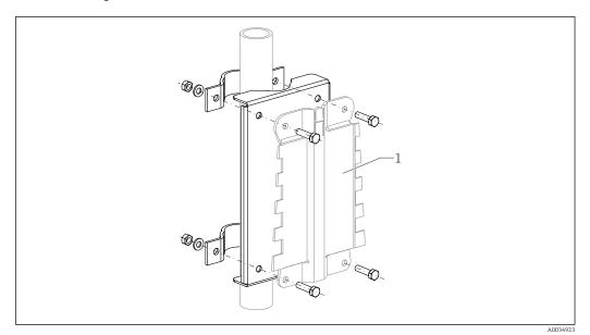
Image: B Mounting plate for mounting the polycarbonate field housing on a post
