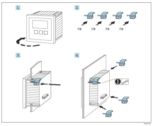
■ 15 Installation of the remote display and operating module
