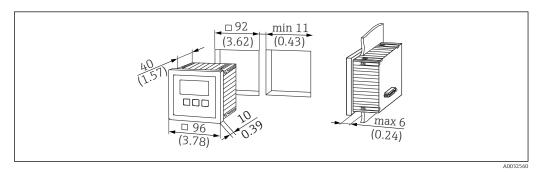
I3 Opening for remote display and operating module. Unit of measurement mm (in)
