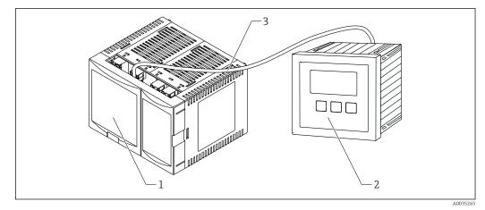
€ 4 Parts of the Prosonic S with remote display and operating module
