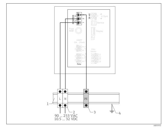
Connection of the power supply in the DIN rail housing 24
