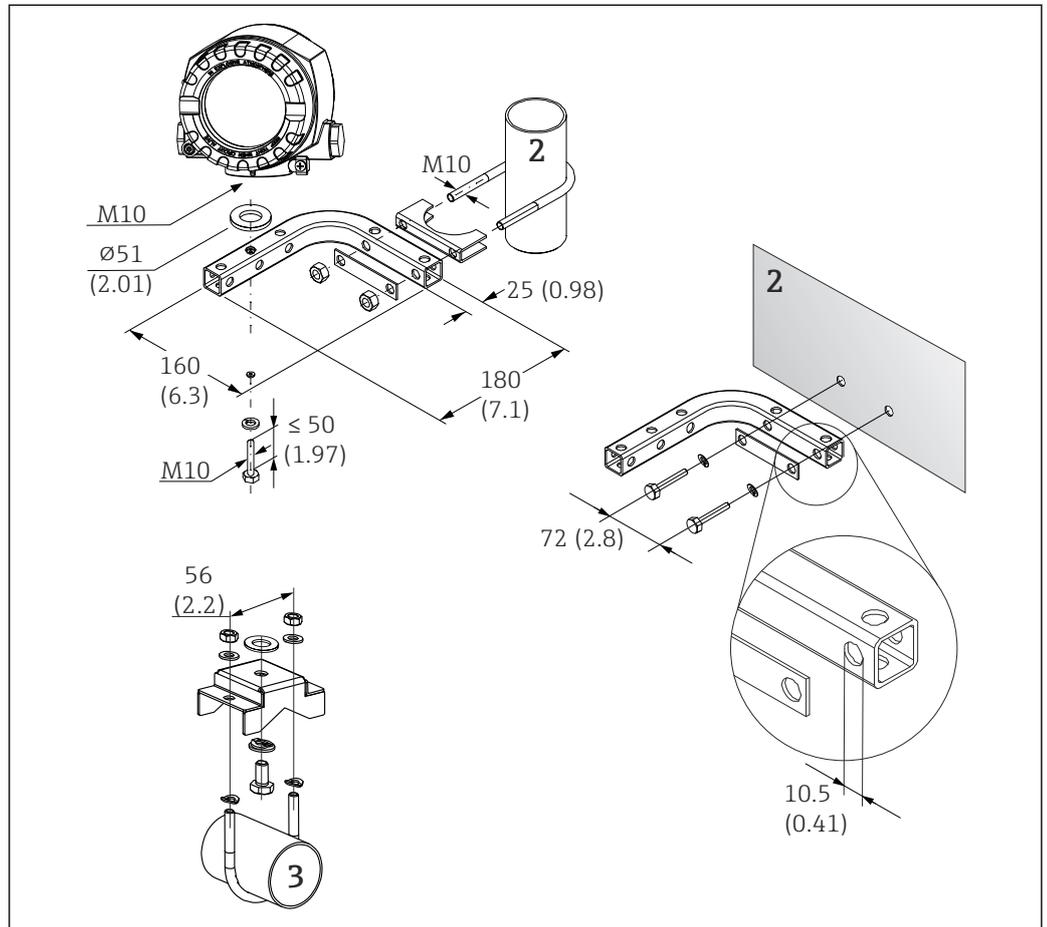
3 Installation of the field transmitter using the mounting bracket, see chapter 'Accessories'. Dimensions in mm (in)
