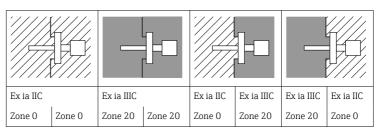
The device is designed for operation in explosive gas or explosive dust atmosphere as shown in the sketch above. In the event of potentially
