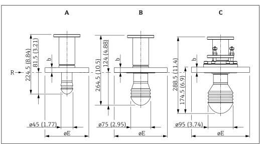
Antenna size; unit of measurement: mm (in)
