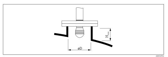
$\emptyset D$  Inner nozzle diameter  $H_{max}$  Maximum nozzle length
