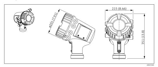
**■** 14 Dimensions of the electronics housing; unit of measurement: mm (in); adapters for cable entries are not taken into account in this drawing.
