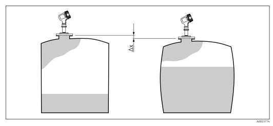
$\blacksquare$  21 Movement  $\Delta x$  of the Gauge Reference Height due to the bulging of the tank shell caused by hydrostatic pressure
