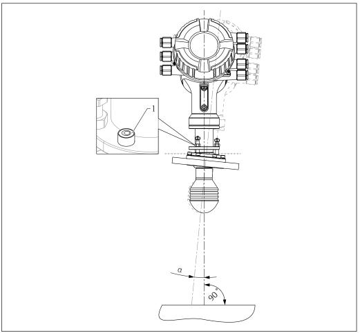
$\blacksquare$  13 Alignment unit of the 100mm(4") antenna
