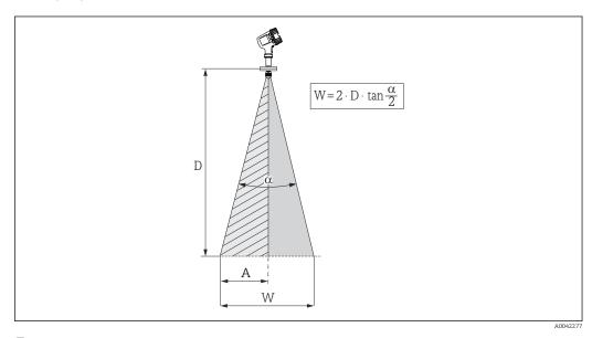
$\blacksquare$  12 Relationship between beam angle a, distance D and beam diameter W. Distance A is the minimum distance to the tank wall (or other installations). Distance A equals the half of beam diameter W
