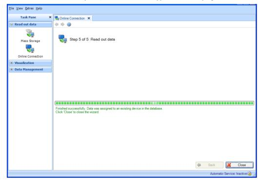
The defined data have now been read out of the device successfully and stored to the database. The stored data have also been successfully deleted from the device memory.
