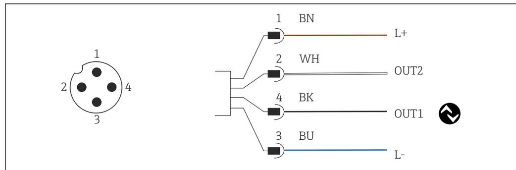
**8** Connection via M12 connector (A-coded)
