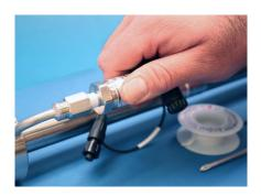
Figure B-9 Replacing pressure sensor
