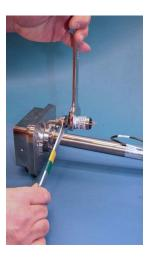
**Figure B-6** Removing the old pressure sensor
