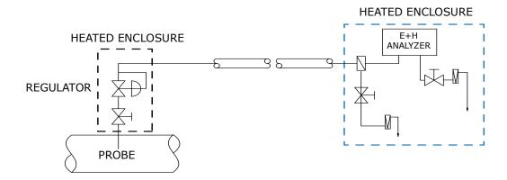
**Figure 4–1** Probe to gas analyzer interface
