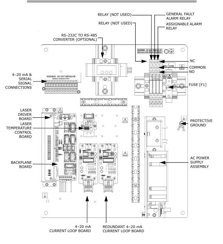
**Figure 1–6** Electronics control board (AC) for single-channel systems (SS500e/SS2000e) with RS-232C to RS-485 converter
