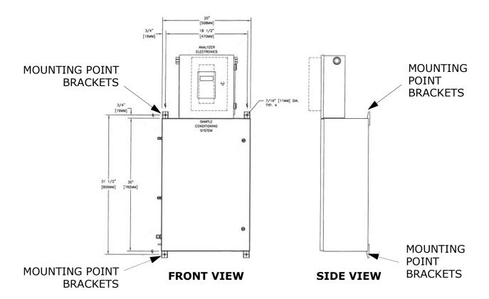
**Figure 3–1** Gas analyzer carrying points/methods
