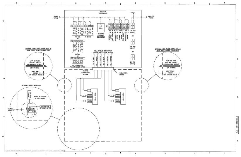
Figure A-10 SS3000e dual stream analyzer system power and signal wiring
