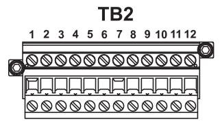
**Figure 3–5** Mating terminal block (TB2) in electronics enclosure for connecting signal cables
