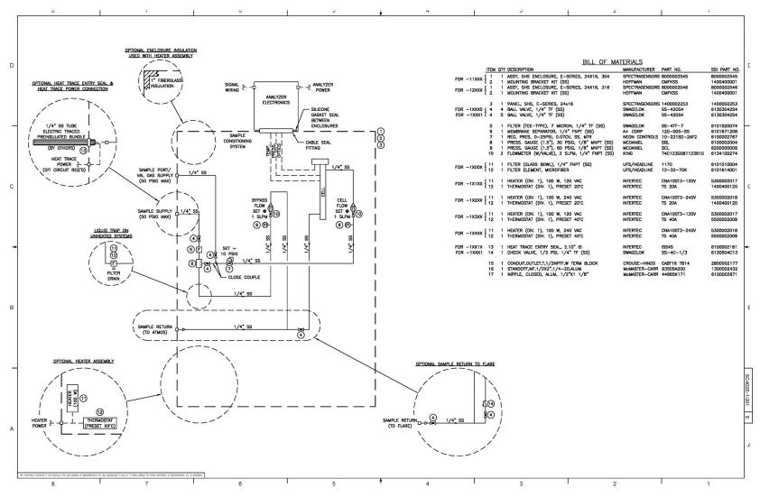
Figure A-2 SS500e/SS2000e analyzer system sample system schematic
