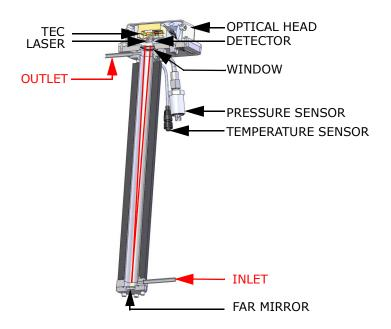
**Figure 1–1** Schematic of a typical laser diode absorption spectrometer
