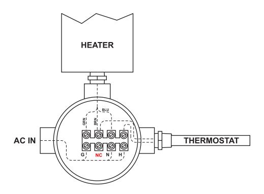
**Figure 3–3** AC connection terminal block for enclosure heater
