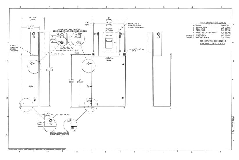
Figure A-4 SS3000e single stream analyzer system outline and mounting dimensions
