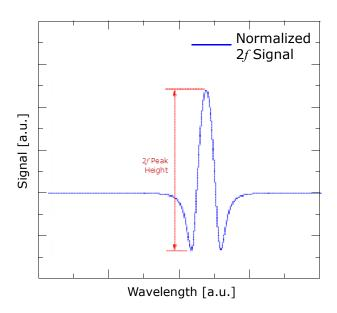
**Figure 1–4** Typical normalized 2f signal; species concentration is proportional to the peak height
