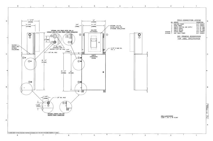
Figure A-1 SS500e/SS2000e analyzer system outline and mounting dimensions
