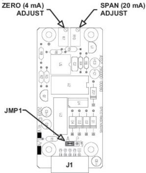
Figure 3-7 4-20 mA output board
