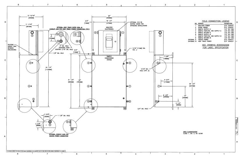
**Figure A-7** SS3000e dual stream analyzer system outline and mounting dimensions
