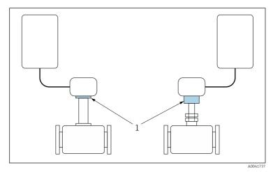
Position of reference point for temperature measurement
