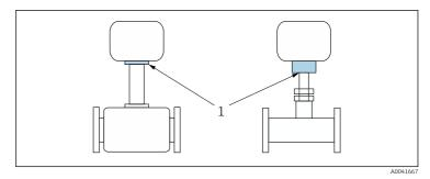
Position of reference point for temperature measurement
