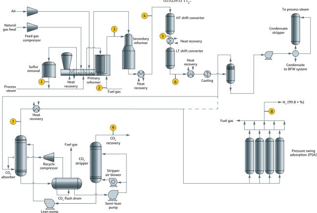
Figure 1: A simplified process diagram showing the main process units for the generation of captive hydrogen inside the battery limits (ISBL) of a modern refinery
