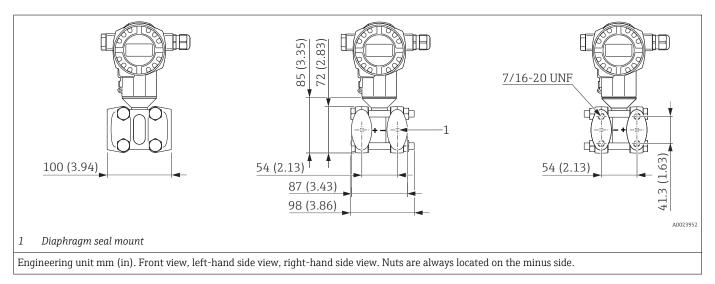
Process connections FMD78 with diaphragm seal
