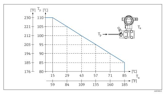
*T<sub>a</sub>* Maximum ambient temperature at the manifold
