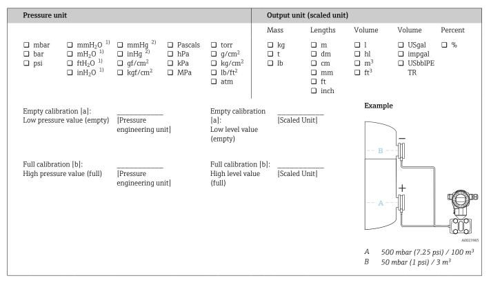
1) The conversion factor for the pressure unit is based on a reference temperature of 4  $^{\circ}C$  (39.2  $^{\circ}F$ ).
