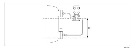
The maximum height difference is dependent on the density of the filling oil and the lowest pressure that is ever allowed to occur at the diaphragm seal on the positive side (empty vessel), see the following illustration:
