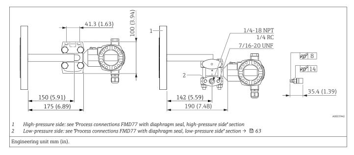
Process connections FMD77 with diaphragm seal
