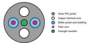
Figure 1. Cross section of a Raman fiber optic cable
