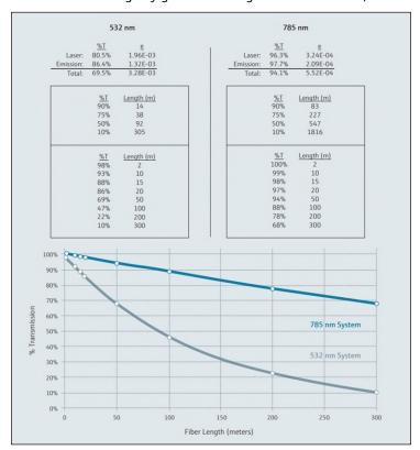
Figure 5. Measured fiber transmission (%T) vs. fiber length
