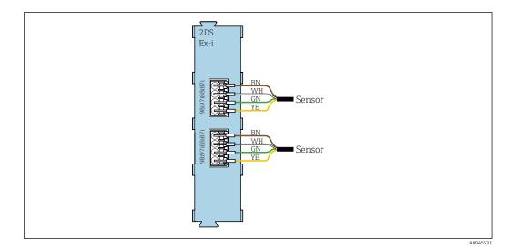
To avoid any mix-up between intrinsically safe and non-intrinsically safe circuits, non-intrinsically safe sensors cannot be operated on a transmitter with intrinsically safe sensor circuits. The corresponding terminals are disabled.
