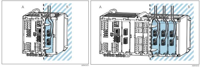
A: Non-intrinsically safe wiring B: Intrinsically safe wiring of sensor communication module 2DS Ex-i
