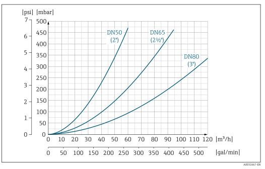
If Pressure loss DN 50 to 80 (2 to 3") for order code for "Design", option C "Fixed flange, constricted measuring tube", 0 x DN inlet/outlet runs"
