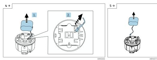
• Take the battery out of the battery compartment (it is still attached, however) and disconnect the battery plug.
