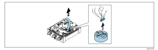
8. Disconnect the plug of the electronics module.
