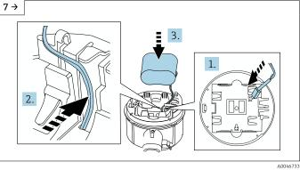
Insert the battery plug and place the cable in the recess of the battery carrier as shown in the graphic. Place the battery in the battery compartment.
