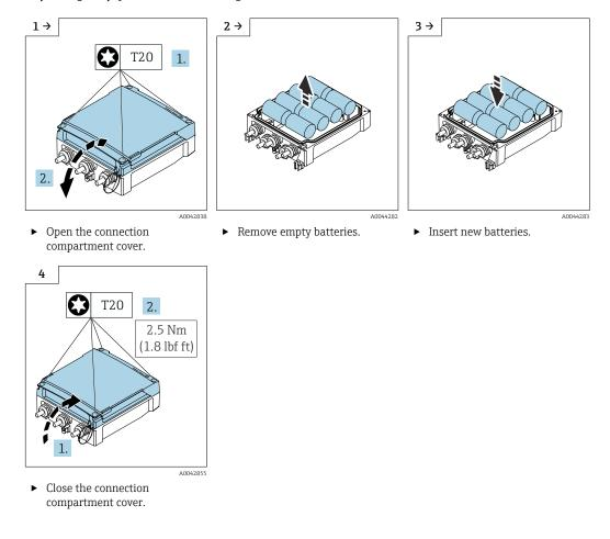
Replacing empty batteries - Promag 800 Advanced
