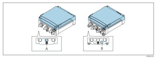
A Plug for the pressure sensor on the housing of the compact transmitter
