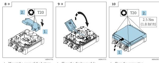
Mount the cover of the battery pack. • Close the display module.
