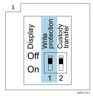
Information regarding the write protection switch is provided on the connection nameplate in the connection compartment cover.
