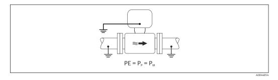
Connect the connection housing of the transmitter or sensor to ground potential via the ground terminal provided for this purpose.
