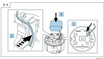
Insert the plug of the battery and place the cable in the slot of the battery carrier, as shown in the graphic. Place battery in battery compartment.
