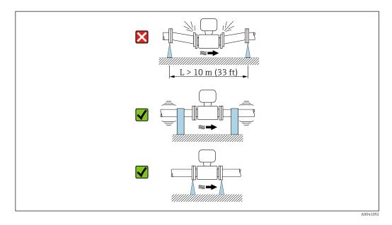
Information on the measuring system's resistance to vibration and shock  $\rightarrow$   $\cong$  105
