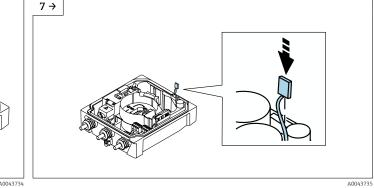
• Plug the buffer capacitor into connector 3.
