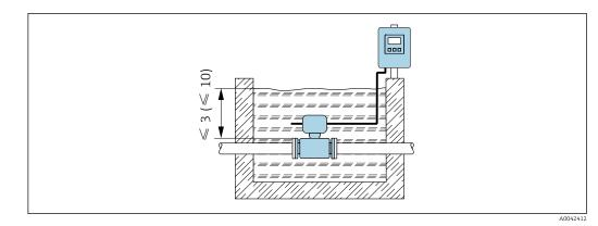
Installation for permanent immersion in water
