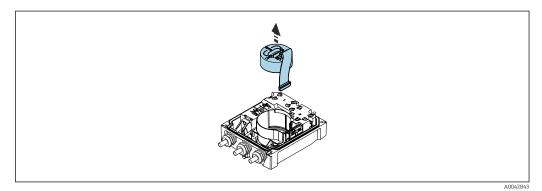
**10.** Remove the electronics module.
