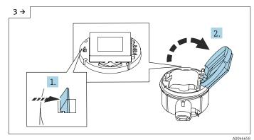
• Open the cover of the electronics carrier.
