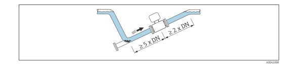
No inlet and outlet runs for devices with the order code for "Design": Option C.
