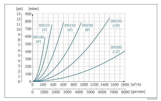
■ 17 Pressure loss DN 100 to 300 (4 to 12") for order code for "Design", option C "Fixed flange, constricted measuring tube", 0 x DN inlet/outlet runs"
