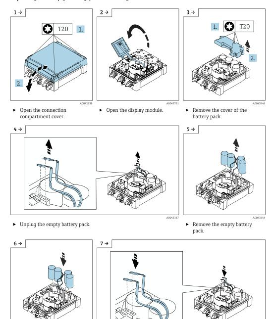
Replacing the empty battery pack - Promag 800 Advanced
