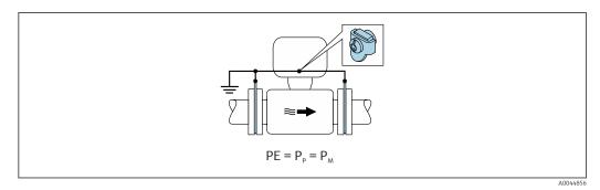
1. Connect the ground disks to the ground terminal of the transmitter or sensor connection housing via the ground cable.
