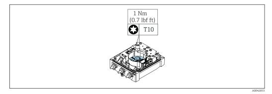
9. Release the screws on the electronics module.
