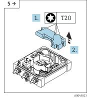
Remove the cover of the battery pack.
