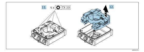
**11.** Loosen the fixing screws of the main electronics module (when reassembling, pay attention to the tightening torque  $\rightarrow \triangleq 41$ ).
