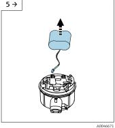
Take the battery out of the battery compartment (it is still attached, however) and disconnect the battery plug.  Now remove the battery from the battery compartment entirely.
