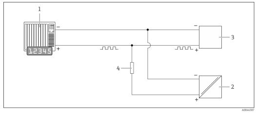
■ 13 Connection example for pulse output (passive)
