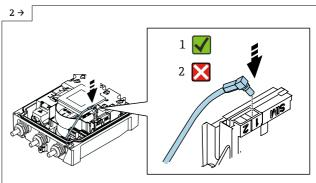
Open the connection compartment cover. ▶ Plug in the antenna connector.
