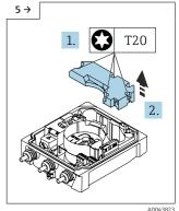
▶ Remove the cover of the battery pack.
