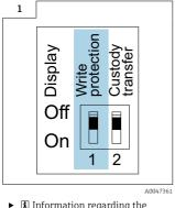
Information regarding the write protection switch is provided on the connection nameplate in the connection compartment cover.
