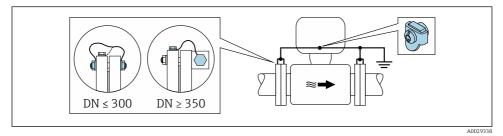
9 Potential equalization via ground terminal and pipe flanges
