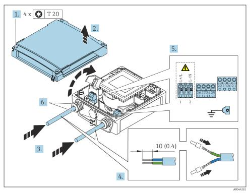
Connecting the supply voltage and Modbus RS485
