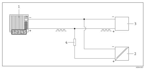
I1 Connection example for pulse output (passive)
