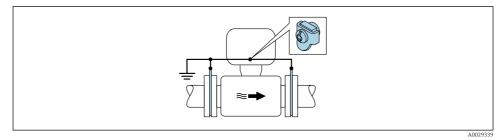
• Potential equalization via ground terminal and ground disks ( $PE = P_{FL} = P_M$ )
