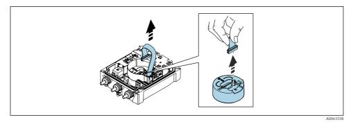
8. Disconnect the plug of the electronics module.
