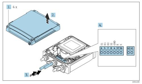
6 Transmitter: main electronics module with terminals
