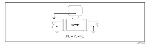
Connect the connection housing of the transmitter or sensor to ground potential via the ground terminal provided for this purpose.
