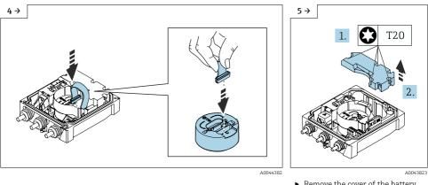
Remove the cover of the battery pack.
