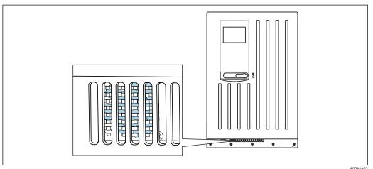
☑ 70 Fan of the cooling module (behind the ventilation grille)
