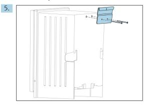
Screw the suspension bracket of the wall holder unit (included in the delivery with the analyzer) onto the analyzer.
