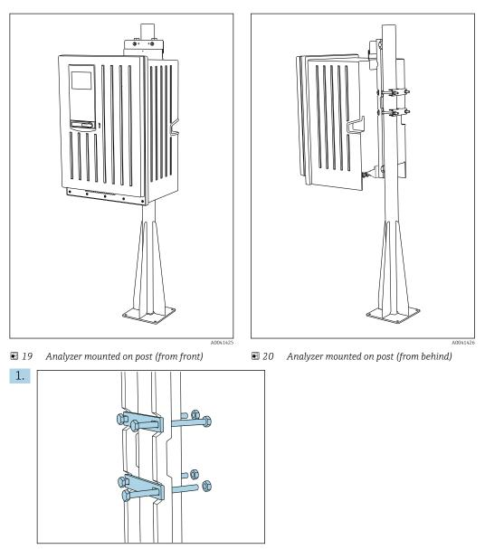
Fit the clamp of the post retainer on the retaining rods and post using the nuts.
