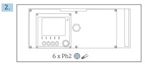
Release the 6 screws on the electronics compartment cover using a Phillips-head screwdriver and fold out the cover towards the front.
