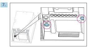
Guide the heated waste hose (left in the graphic) and the heated sample hose (right in the graphic) through the cable glands indicated.
