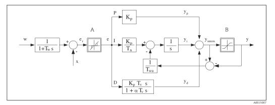
■ 65 Block diagram of the controller structure
