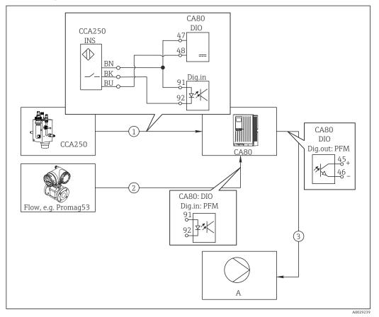
■ 55 Example of chlorine control with feedforward control
