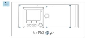
Release the 6 screws on the electronics compartment cover using a Phillips-head screwdriver and fold out the cover towards the front.
