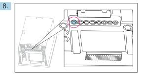
Guide the power supply cable, which is provided by the customer at the installation location, through the cable gland indicated.
