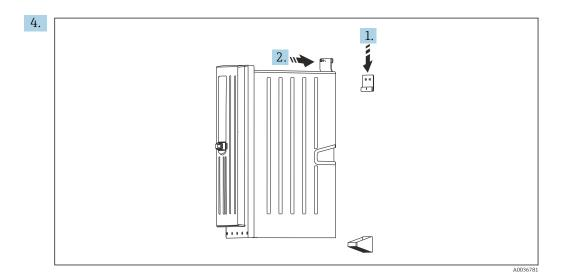
Hook the analyzer into the wall holder unit (1).
