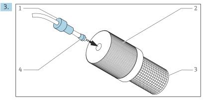
Mounting the suction strainer (supplied) on the sample hose 🖸 54
