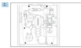
Release the 5 screws on the carrier board using a Torx screwdriver (T25).
