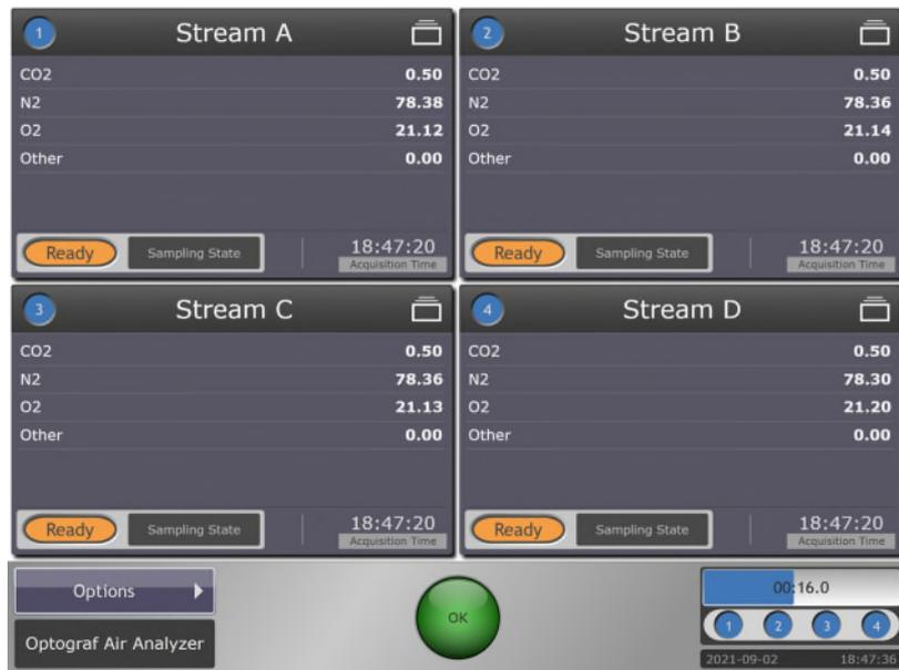
Figure 5. Raman RunTime's main view in a Rxn5 four channel analyzer
