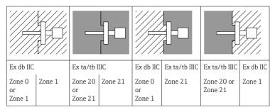
The device is designed for operation in explosive gas or explosive dust atmosphere as shown in the sketch above. In the event of potentially explosive gas-air and dust-air mixtures occurring simultaneously: Suitability requires further assessment.
