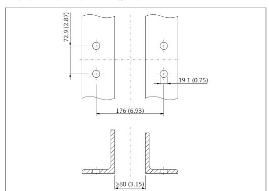
Example of mounting with angle bracket (supplied by customer)
