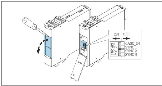
₽8 Visualization of the operating elements (DIP switches)
