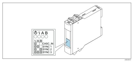
**₽** 7 Arrangement of the display LEDs
