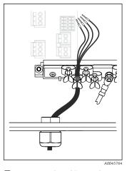
**№** 38 Press the cable into the grounding clamp
