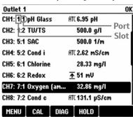
**№** 6 Slot and port assignment on the display
