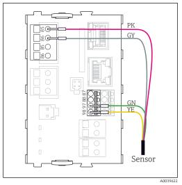
$\blacksquare$  45 Memosens sensors without additional supply voltage
