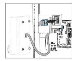
5. Pull the display cable through the hole in the middle, and place the display from the outside through the four holes drilled for this purpose, ensuring that the torx screws have been unscrewed to the last half turn but are still in place. Ensure that the rubber frame (seal, highlighted blue) does not become damaged and is properly positioned on the surface of the door.
