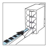
Insert the cable until the limit stop.
