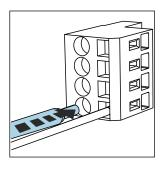
Insert the cable until the limit stop.
