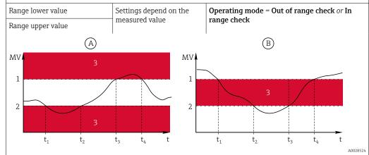
🖩 90 Range monitoring outside (A) and within (B) a range (without hysteresis and switch-on delay)
