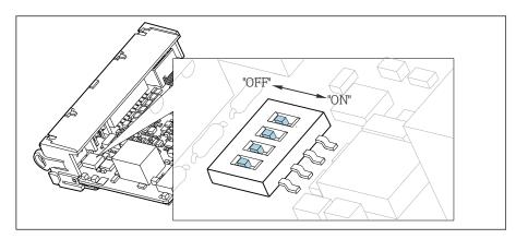
■ 76 DIP switch for internal termination
