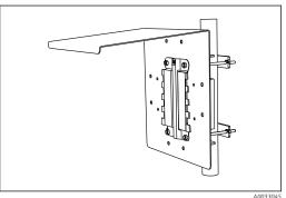
1. Place the device on the mounting plate.
