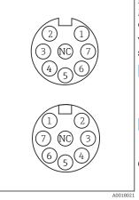
**■** 50 *M12 assignment Top:* socket Bottom: plug (top view in each case)
