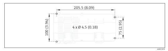
■ 13 Drilling pattern for wall mounting in mm (in)
