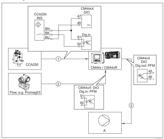
$\blacksquare$  87 Example of chlorine control with feedforward control
