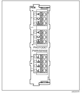
■ 47 Sensors with and without additional supply voltage at sensor module 2DS
