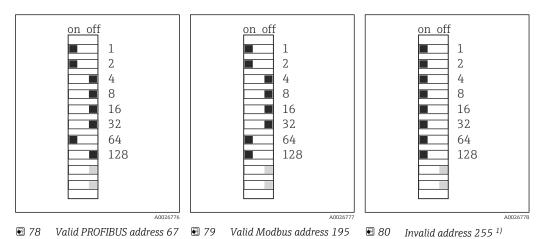
1) Order configuration, software addressing is active, software address configured at the factory: PROFIBUS 126, Modbus 247
