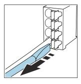
• Remove the screwdriver (closes the terminal).
