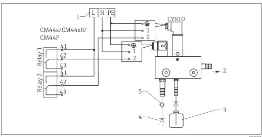
€ 65 Connecting the CYR10 injector cleaning unit
