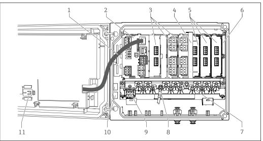
₩ 3 Example of a field device with sensor communication module type 2DS Ex-i and open display cover (without wiring)
