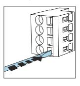
Press the screwdriver against the clip (opens the terminal).
