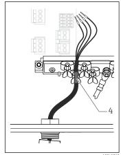
Connect the cable to the grounding clamp
