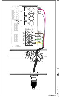
₩ 49 M12 plug-in connector (e.g. at sensor module)
