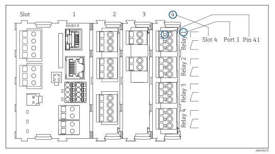
$\blacksquare$  7 Creating a terminal diagram using the example of the NO contact (terminal 41) of a relay
