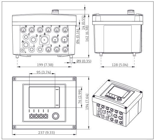
₽8 Dimensions of field housing in mm (inch)
