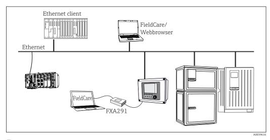
■ 31 Modbus TCP or EtherNet/IP or PROFINET
