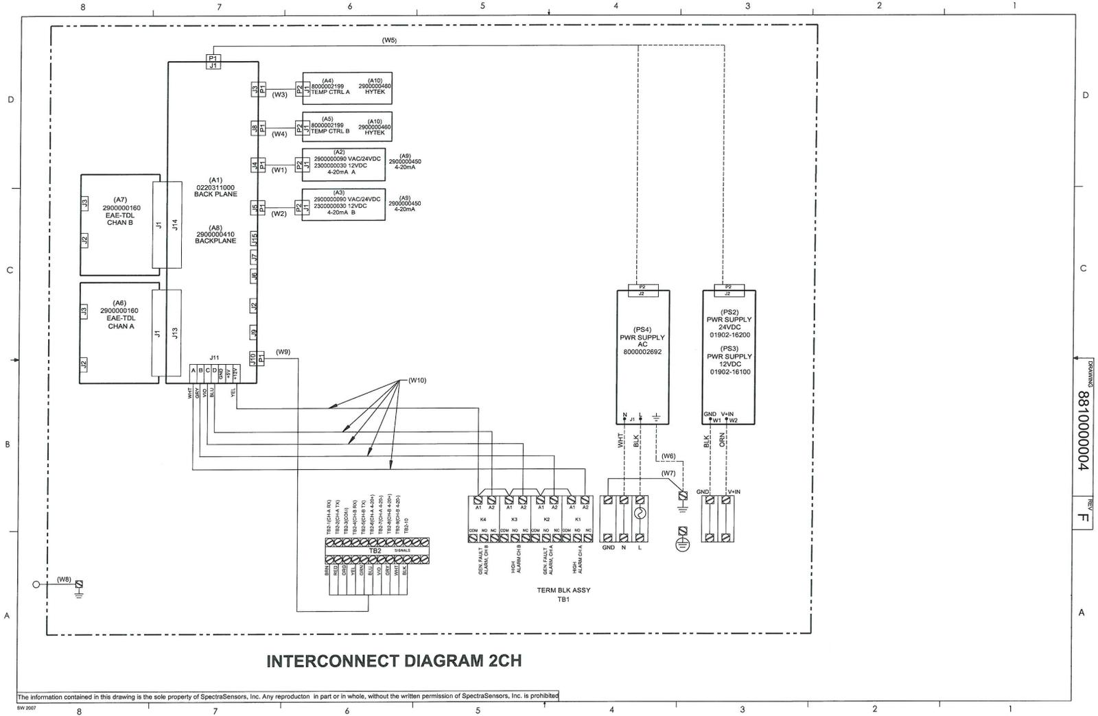
Figure A-7 Interconnect diagram for dual-channel system (SS3000)
