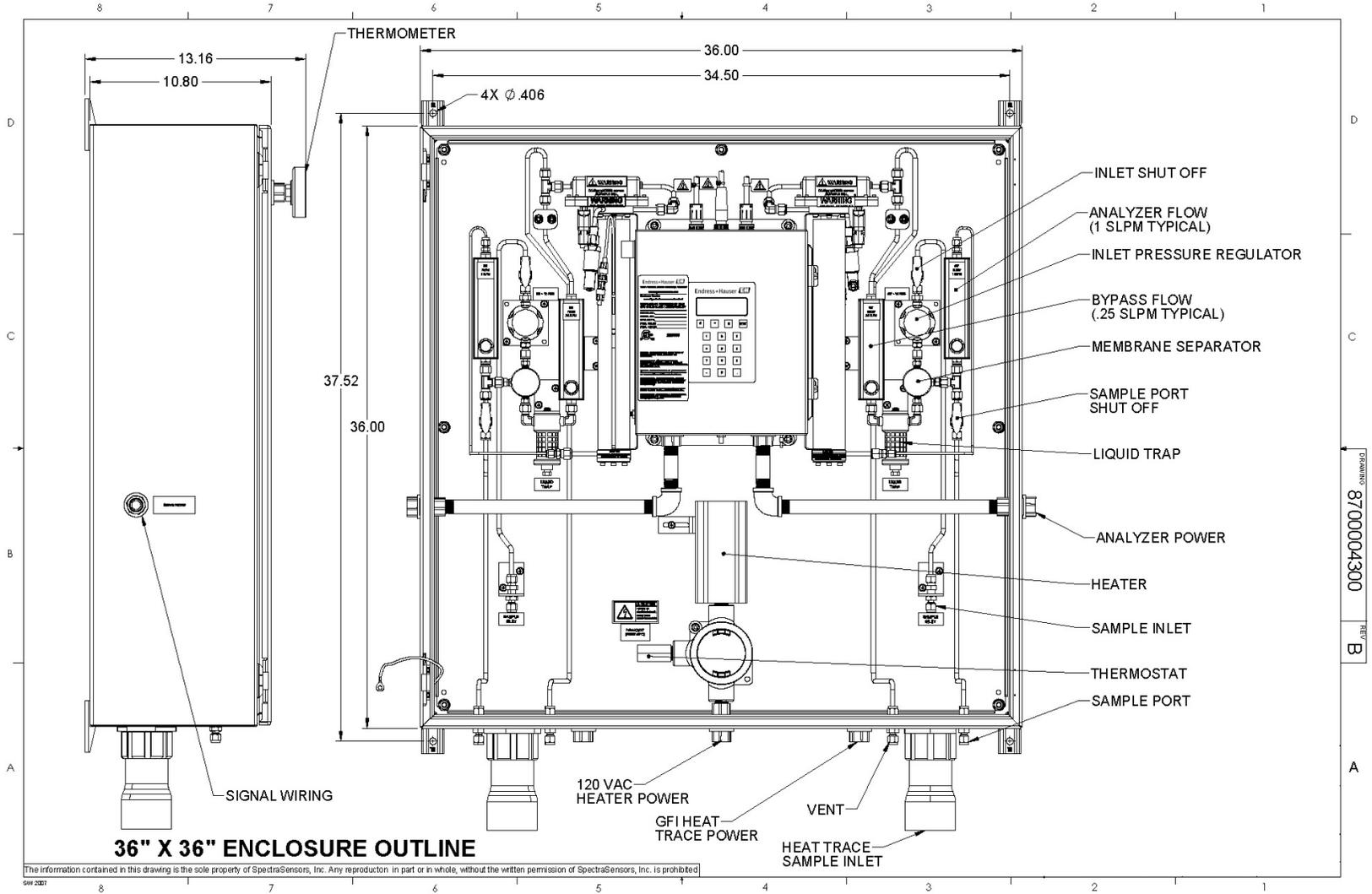
**Figure A-5** Drawing of typical full-featured dual-channel, dual-stream SCS (SS3000) in a 36 X 36 enclosure
