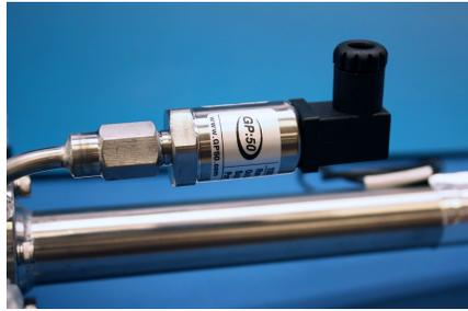
**Figure B-10** Newly installed pressure sensor positioning
