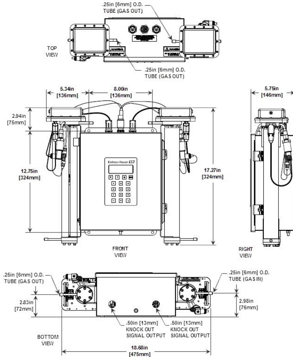
**Figure A-2** SS3000 0.8 m/0.8 m cells (H<sub>2</sub>O/H<sub>2</sub>O) outline and mounting dimensions
