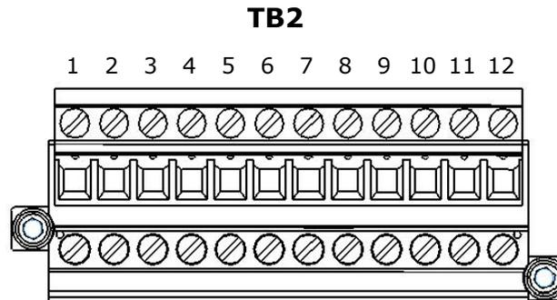
**Figure 3-4** Mating terminal block (TB2) in electronics enclosure for connecting signal cables
