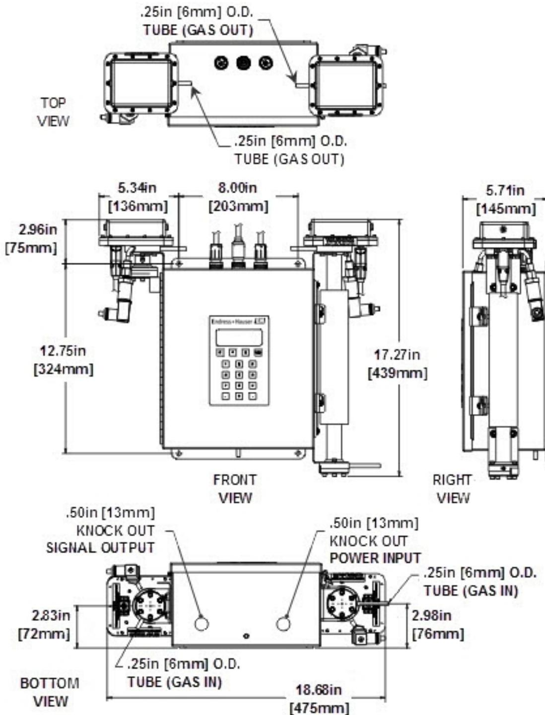
**Figure A-1** SS3000 0.8 m/0.1 m cells (H<sub>2</sub>O/ CO<sub>2</sub>) outline and mounting dimensions
