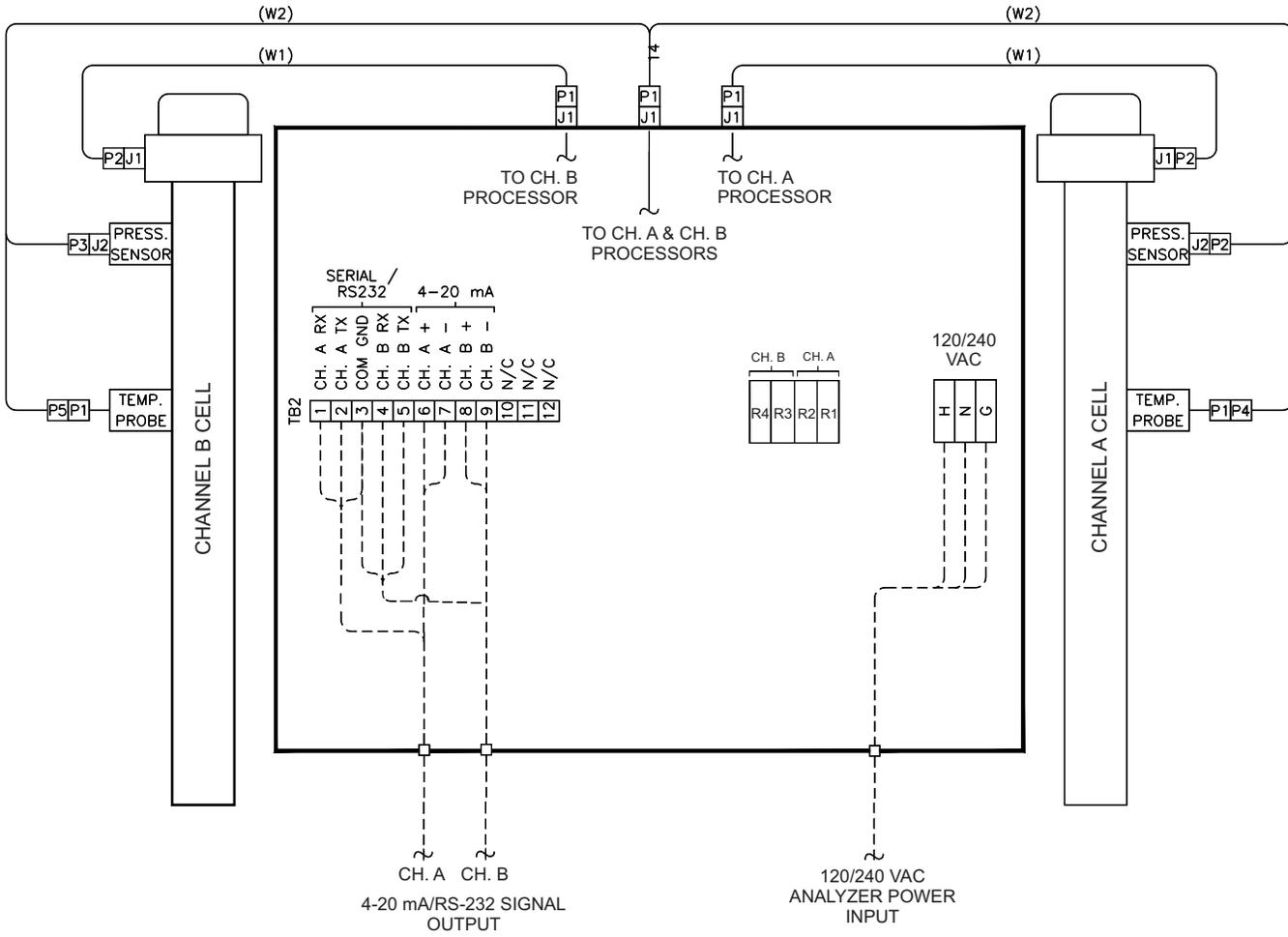
Figure A-6 Electrical schematic for SS3000
