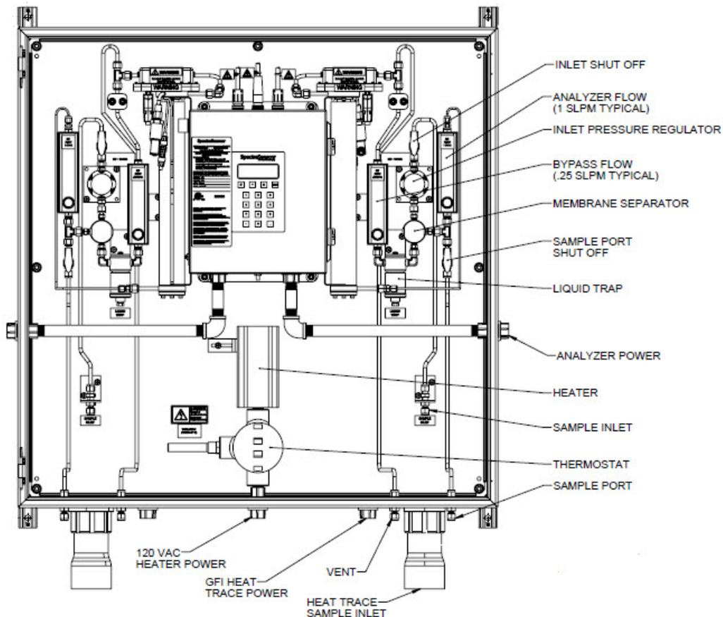
**Figure 4-1** Typical full-featured, single-channel SCS (SS3000) on a panel
