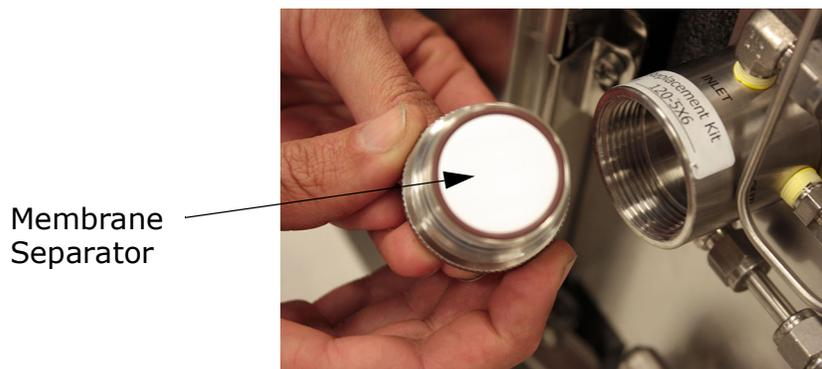
**Figure B-11** Inspecting the membrane separator filter
