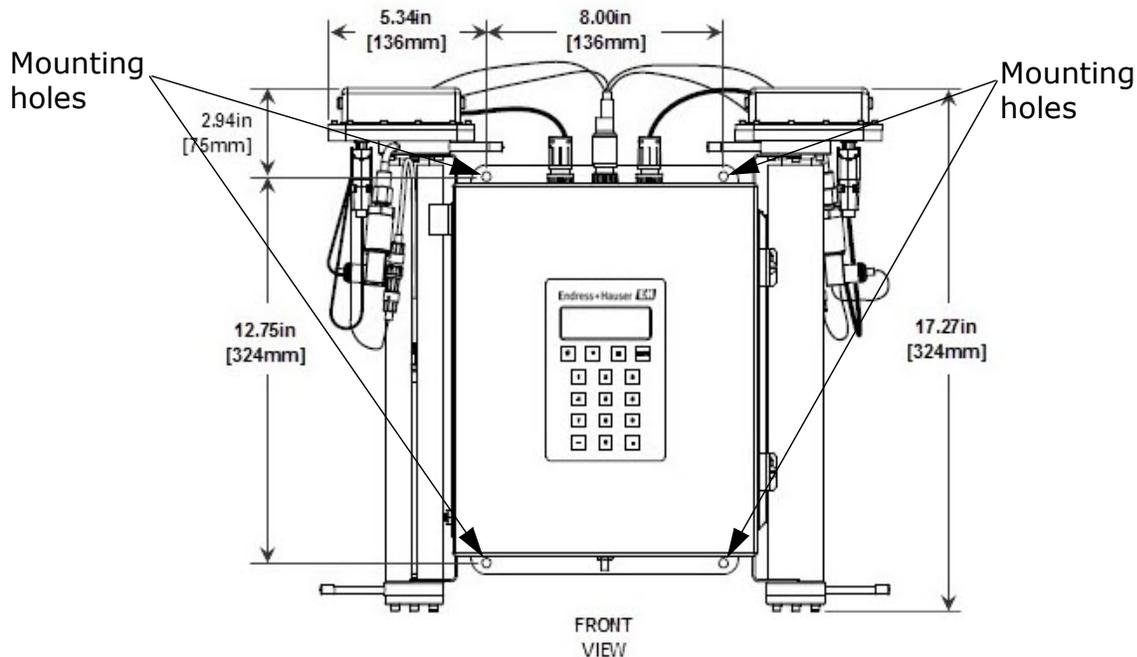
**Figure 3-1** SS3000 TDLAS Gas Analyzer mounting holes
