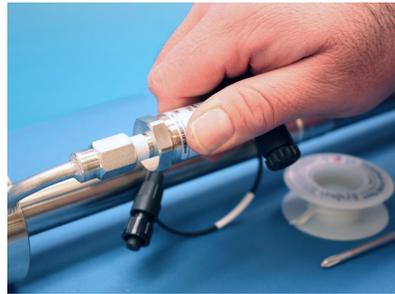
**Figure B-9** Replacing pressure sensor
