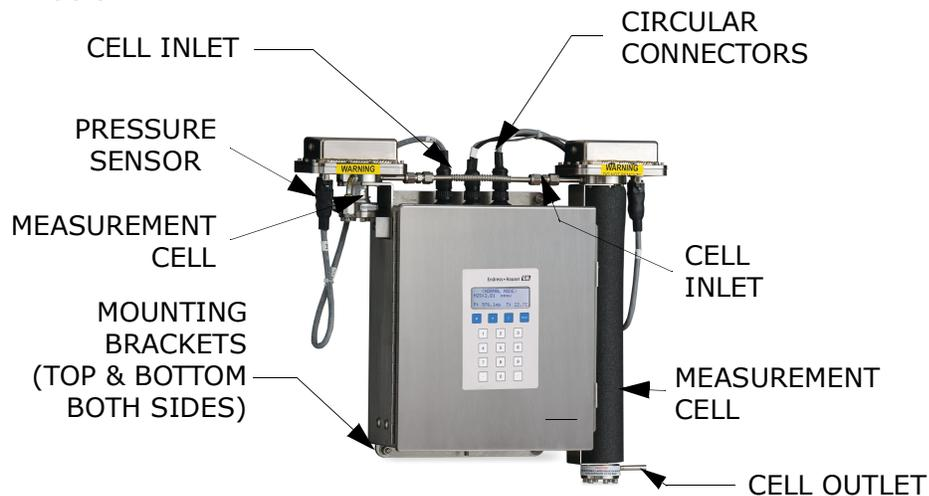
**Figure B-4** Analyzer component locations
