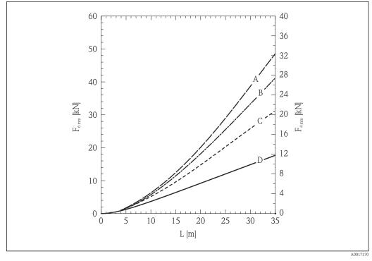
$\blacksquare$  5 Silica sand in metal silo with smooth walls; tensile load as a function of level L for rope diameters 6 mm (0.24 in) and 4 mm (0.16 in)
