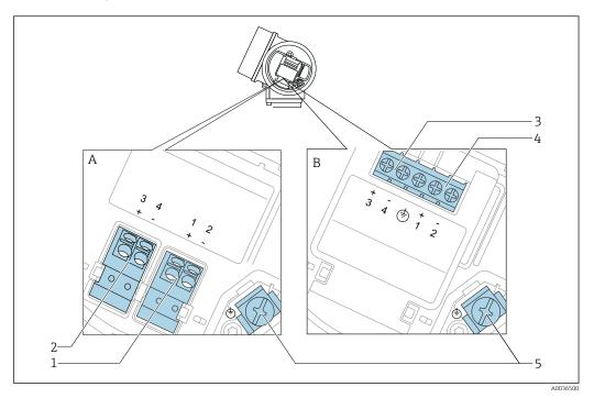
■ 18 Terminal assignment 2-wire: 4-20 mA HART, 4-20 mA
