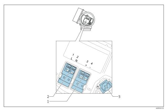
22 Terminal assignment 4-wire: 4-20 mA HART (90 to 253  $V_{AC}$ )
