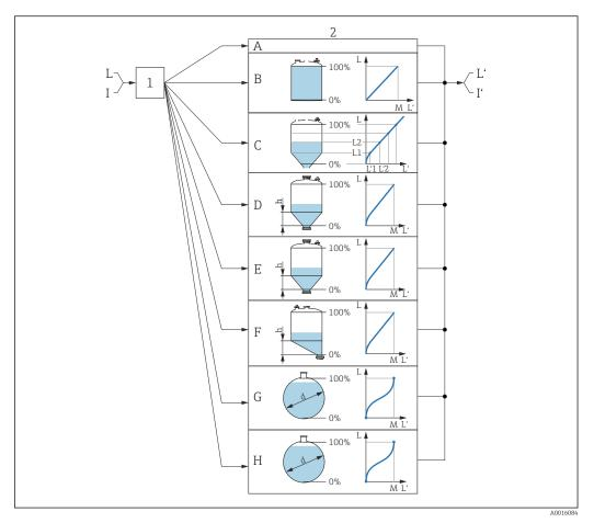
Linearization: Conversion of the level and, if applicable, interface into a volume or a weight; the **■** 52 conversion depends on the vessel shape
