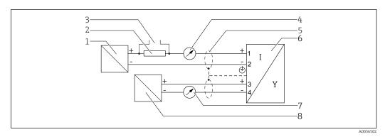
🗷 19 Block diagram 2-wire: 4-20 mA HART, 4-20 mA
