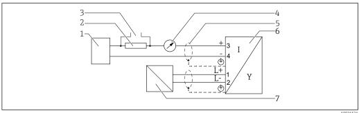
Block diagram 4-wire: 4-20 mA HART (10.4 to 48  $V_{DC}$ )
