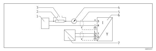
$\blacksquare$  23 Block diagram 4-wire: 4-20 mA HART (90 to 253  $V_{AC}$ )
