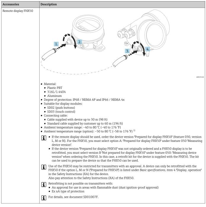
1) This range is valid if option JN "Ambient temperature transmitter -50 °C (-58 °F)" has been selected in ordering feature 580 "Test, Certificate". If the temperature is permanently below -40 °C (-40 °F), failure rates may be increased.
