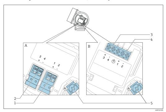
■ 16 Terminal assignment 2-wire: 4-20 mA HART, switch output
