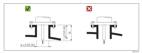
Length of the centering rod or the rigid part of the rope probe
