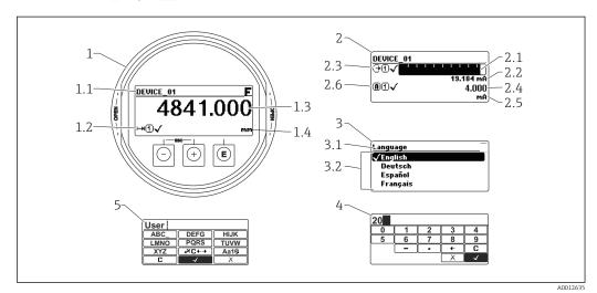
■ 35 Appearance of the display and operation module for on-site operation
