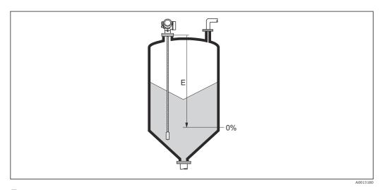
■ 47 Empty calibration (E) for level measurements in bulk solids.
