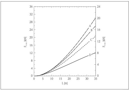
**₽** 7 Wheat in metal silo with smooth walls; tensile load as a function of level L for rope diameters 6 mm (0.24 in) and 4 mm (0.16 in)
