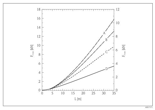
**№** 6 Polyethylene pellets in metal silo with smooth walls; tensile load as a function of level L for rope diameters 6 mm (0.24 in) and 4 mm (0.16 in)
