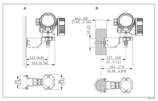
■ 12 Mounting the electronics housing with the mounting bracket. Unit of measurement mm (in)
