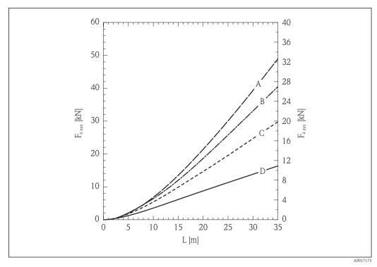
$\blacksquare$  8 Cement in metal silo with smooth walls; tensile load as a function of level L for rope diameters 6 mm (0.24 in) and 4 mm (0.16 in)
