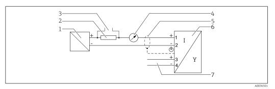
🖪 17 🛮 Block diagram 2-wire: 4-20 mA HART, switch output
