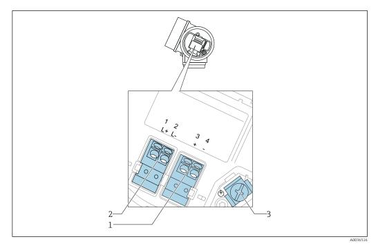
Terminal assignment 4-wire: 4-20 mA HART (10.4 to 48  $V_{DC}$ )
