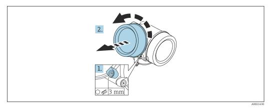
1. Loosen the screw of the securing clamp of the electronics compartment cover using an Allen key (3 mm) and turn the clamp 90 ° counterclockwise.
