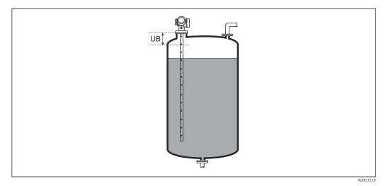
■ 43 Blocking distance (UB) for liquid measurements
