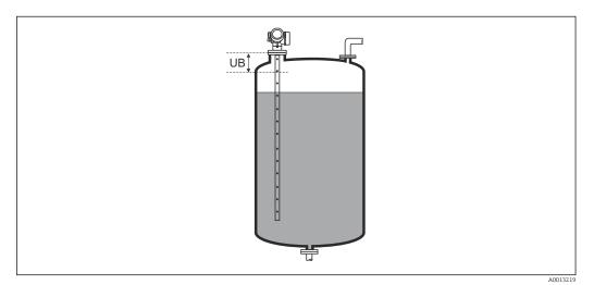
■ 46 Blocking distance (UB) for liquid measurements
