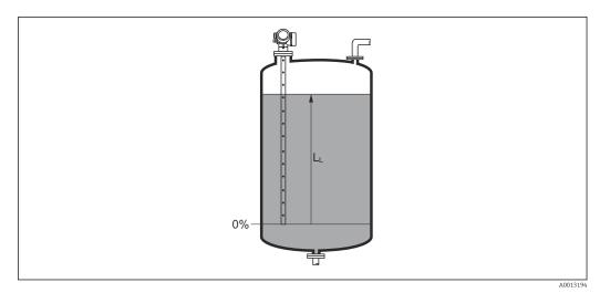
■ 41 Level in case of liquid measurements
