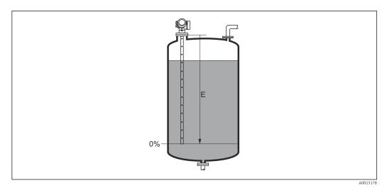
■ 39 Empty calibration (E) for level measurements in liquids
