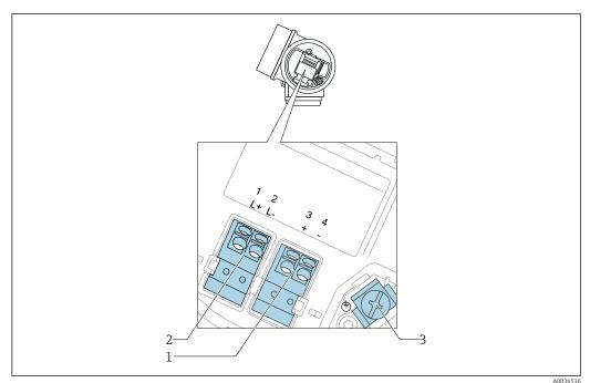
$\blacksquare$  13 Terminal assignment 4-wire: 4-20 mA HART (10.4 to 48  $V_{DC}$ )
