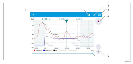
🖪 30 Envelope curve display (sample) in SmartBlue for Android
