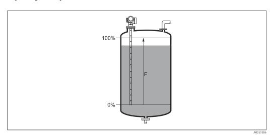
$\blacksquare$  40 Full calibration (F) for level measurements in liquids
