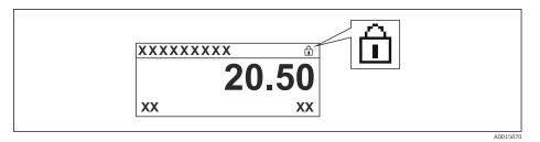
If the hardware write protection is disabled: No option is displayed in the **Locking status** parameter. On the local display, the 🛍-symbol disappears from in front of the parameters in the header of the operational display and in the navigation view.
