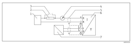
$\blacksquare$  14 Block diagram 4-wire: 4-20 mA HART (10.4 to 48  $V_{DC}$ )
