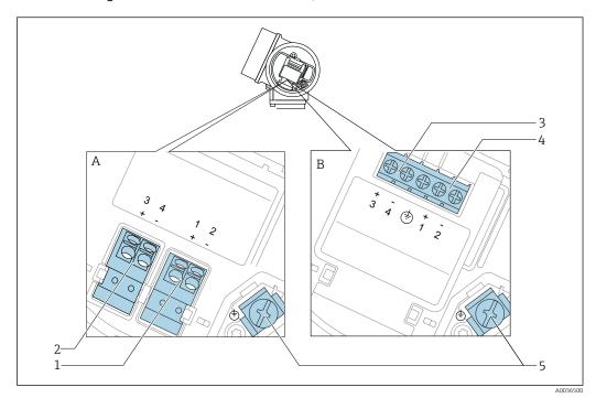
■ 11 Terminal assignment 2-wire: 4-20 mA HART, 4-20 mA
