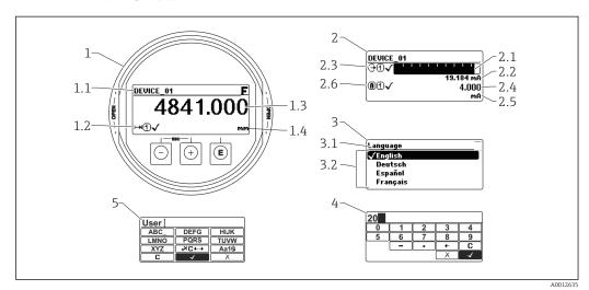
28 Appearance of the display and operation module for on-site operation
