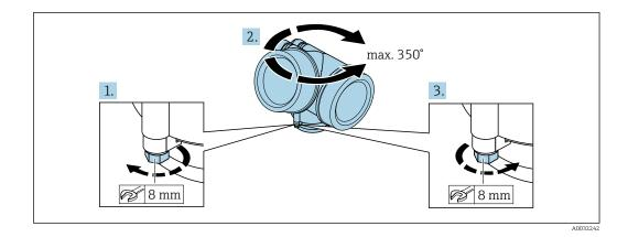
1. Unscrew the securing screw using an open-ended wrench.
