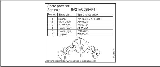
**■** 36 Example for spare part nameplate in the connection compartment cover
