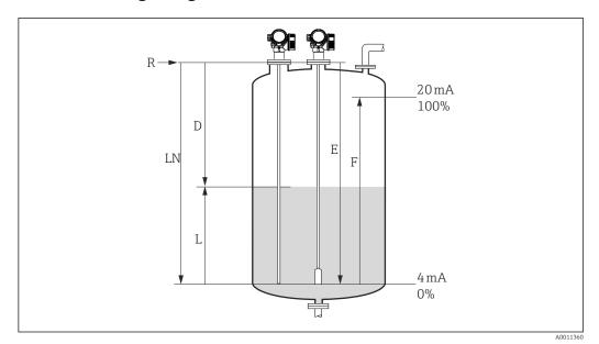
$\blacksquare$  33 Configuration parameters for level measurement in liquids
