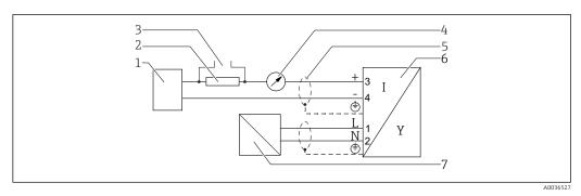
$\blacksquare$  16 Block diagram 4-wire: 4-20 mA HART (90 to 253  $V_{AC}$ )
